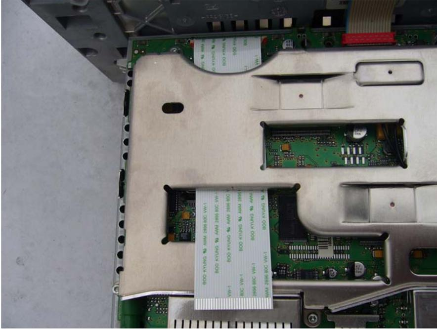
**Connected FTC Cable as picture.**
