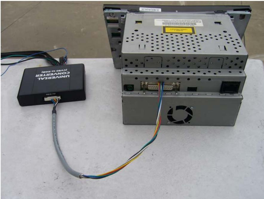
Connect RGB connector with picture equally. Do not harm RGB cable and check each cable without pressured.
