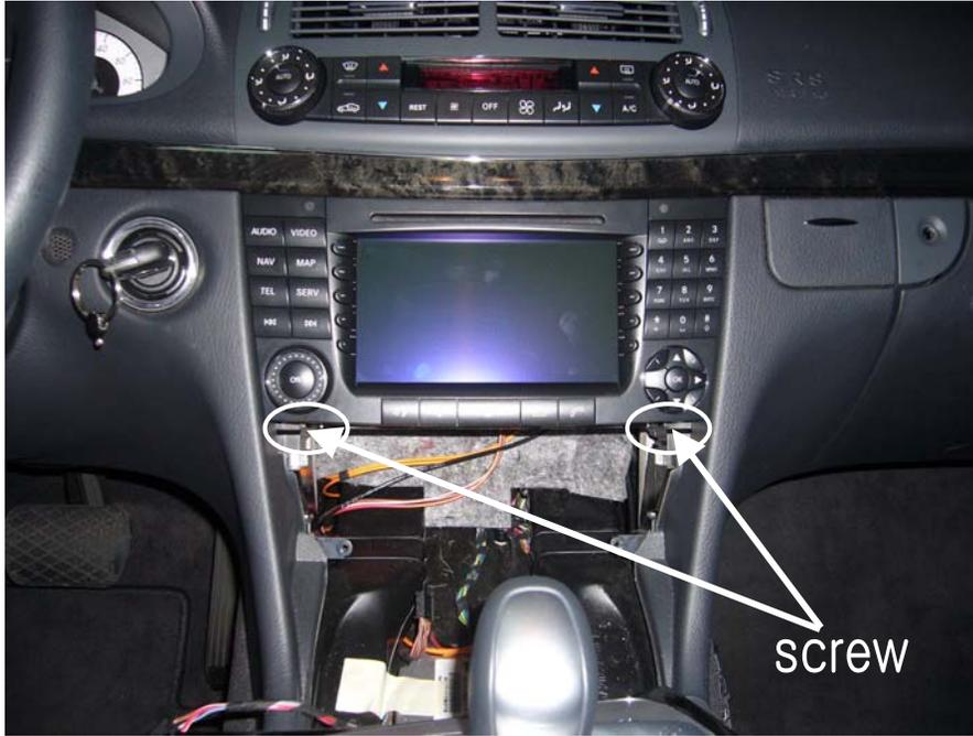
**Screw location for disassembling**
