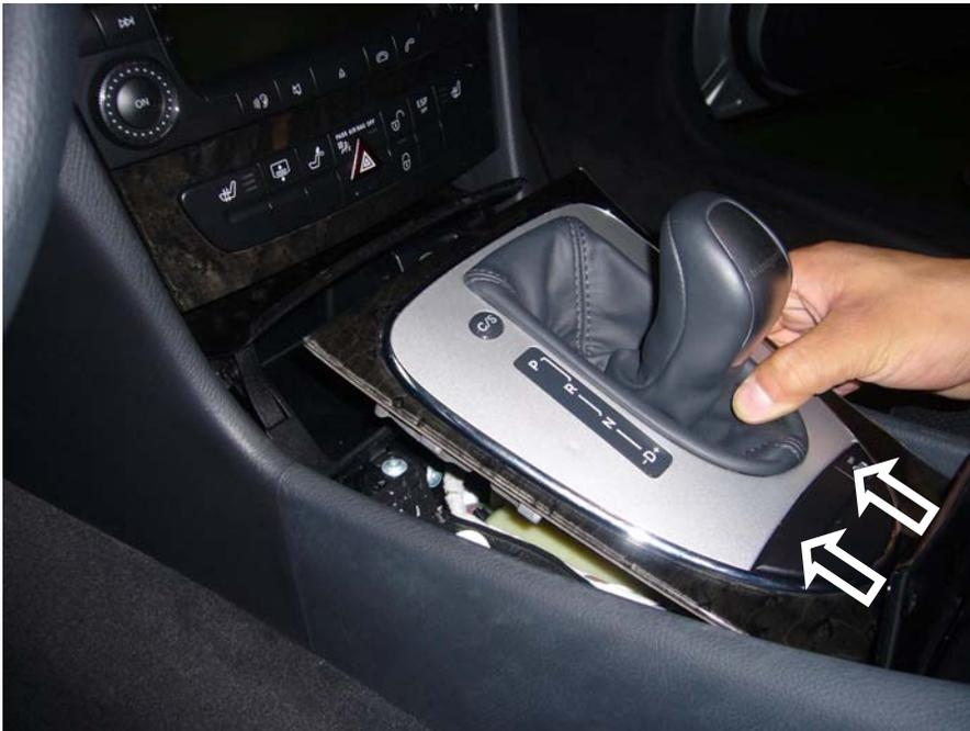
**Release (2<sup>nd</sup> -step) gear-box by hands as arrow direction**
