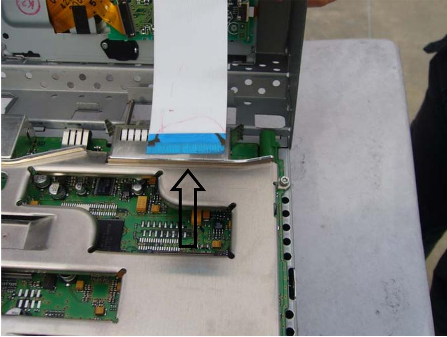
Release FTC cable as arrow direction
