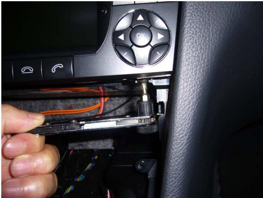
**Release the screw with picture equally**
